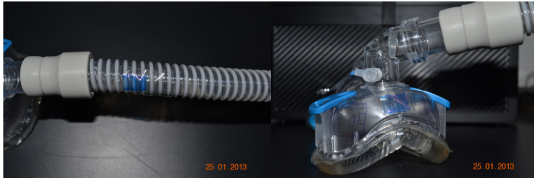
Figure 4: Contaminated surfaces (marked blue) in the hose (left) and the mask (right).
